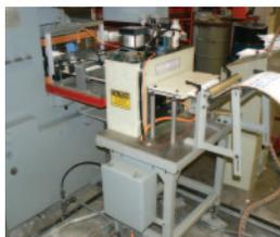
The Registry Feed is a microprocessor controlled, servo driven electronic roll feed. Feed lengths are programmed directly from the remote console for accurate and consistent blanks stroke after stroke.
